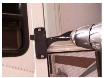
Drill one hole in the latch handle (3/32" bit) being careful to allow room for the retaining latch to be able to grab the release handle, then drill another hole at the top of the plastic door slide stop/handle. (Note: do not drill a hole in the sliding cover, but the cover stop/handle as pictured below).
