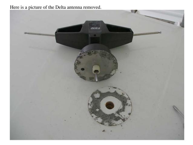
This shows the thickness of the gel-coat (1/4) and the plywood (3/4) the hole is  $1\frac{1}{4}$  in diameter. It was very hard to remove this old sealant.
