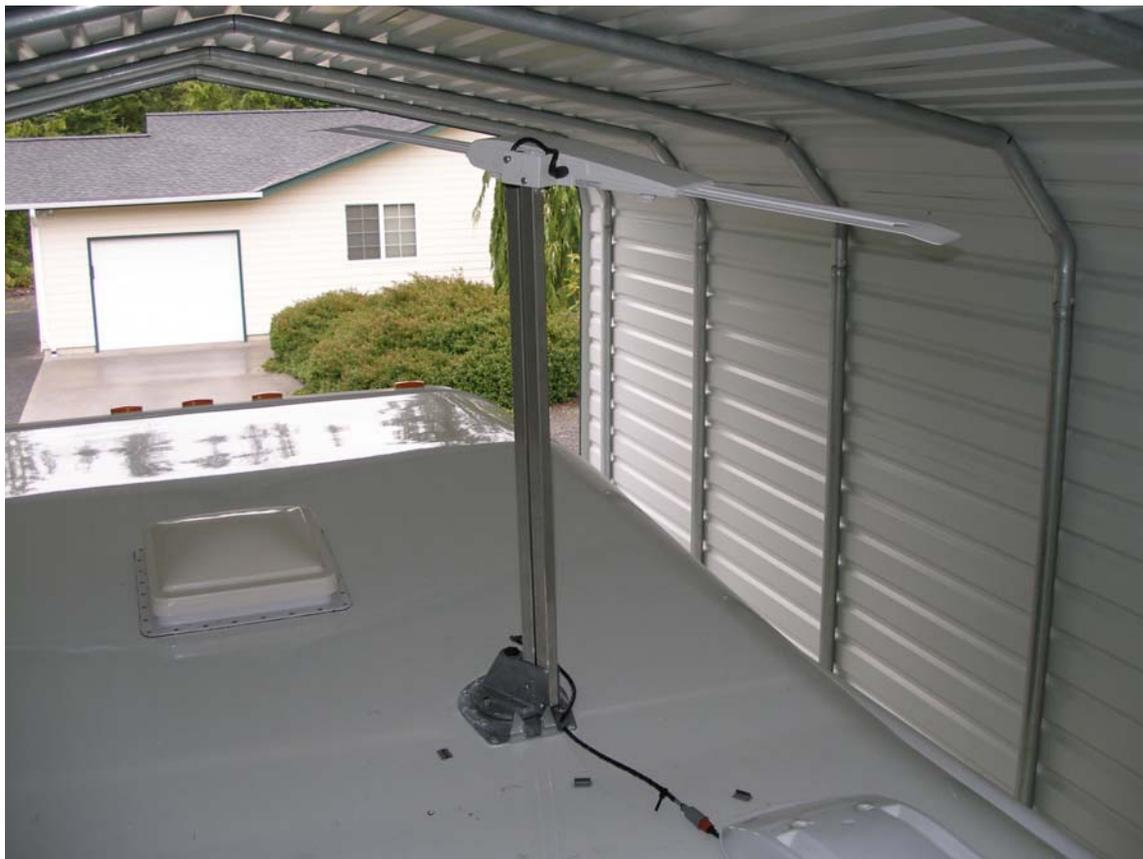
This shows placement of antenna in the stowed position.
