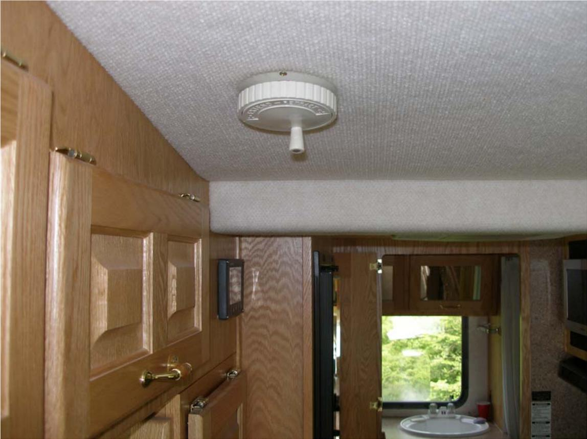
Here is a picture that shows how to remove the handle using a 3/32" Hex wrench.
