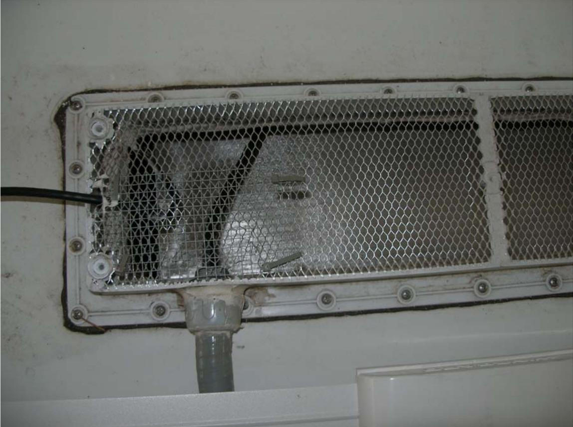
This shows the antenna cable clamped down, I still have to remove the old “stick on” cable clamps from the roof as they are broken anyway. The grey and red connection shown is filled with Permatex (brand) Dielectric grease as are all the “F” type connectors, Winegard states this is not necessary but my experience says otherwise. I also wrapped the cable with 3M (brand) T88 electrical tape to prevent deterioration from UV.
