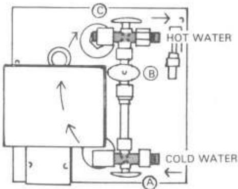
The positioning of valves (A,B,C) for use of water heater. This allows cold water to go thru heater and come out as hot water. (See Shaded Area)
