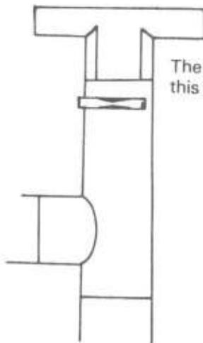
The three drain valves should appear like this when closed.
