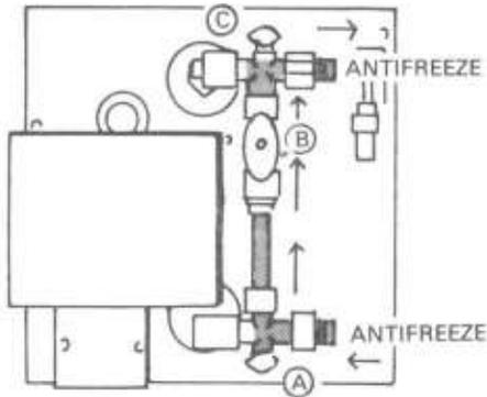
The positioning of the valves (A,B,C) when winterizing with antifreeze. This allows antifreeze to go thru cold water pipe, thru bypass and out thru hot water pipe. (See shaded area.) Antifreeze will not go thru heater if in this position. You should not run antifreeze thru your heater as the tank will "trap" the taste of the antifreeze for summer use.
