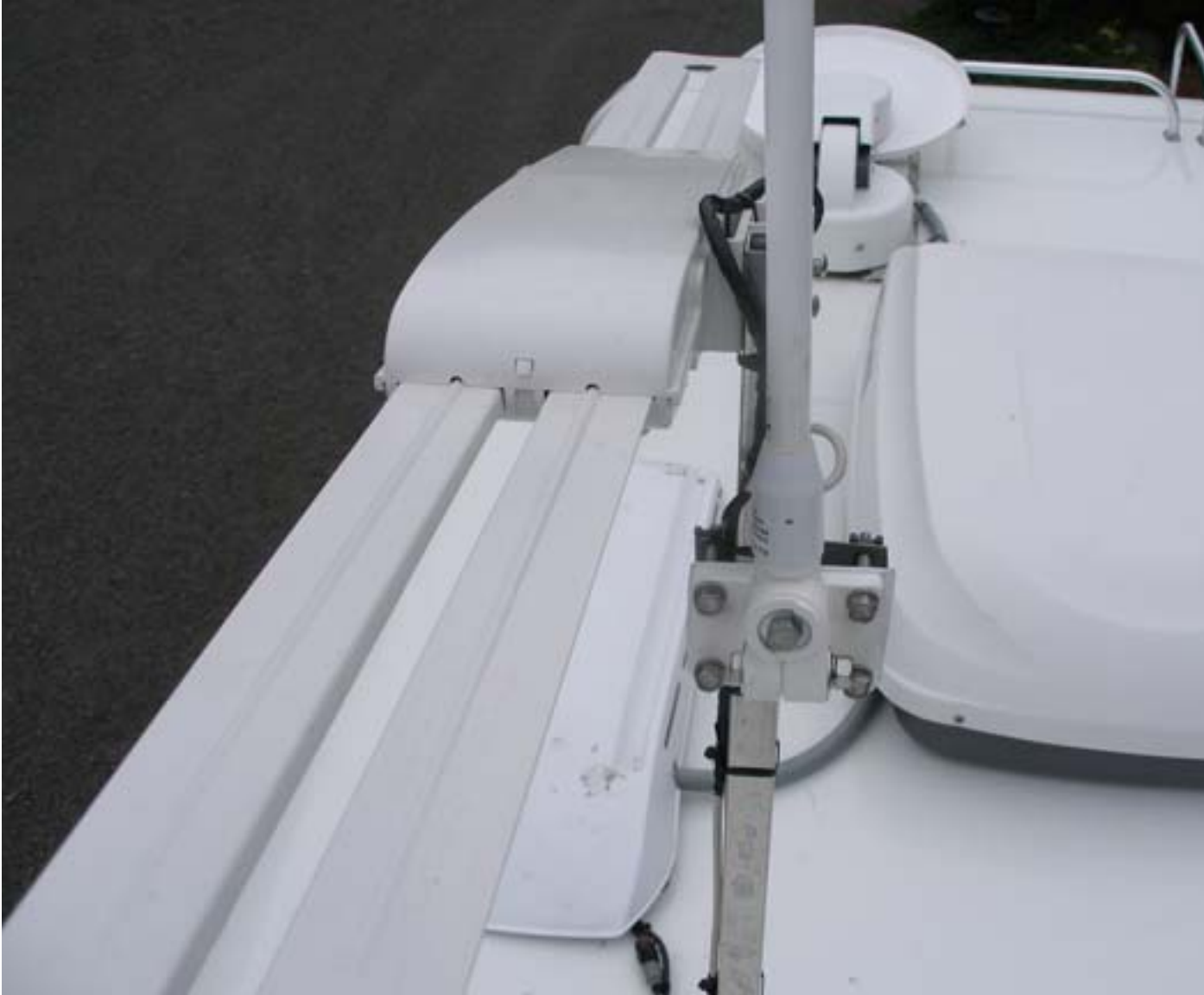
5: Close up of antenna mounting, fully adjustable.
