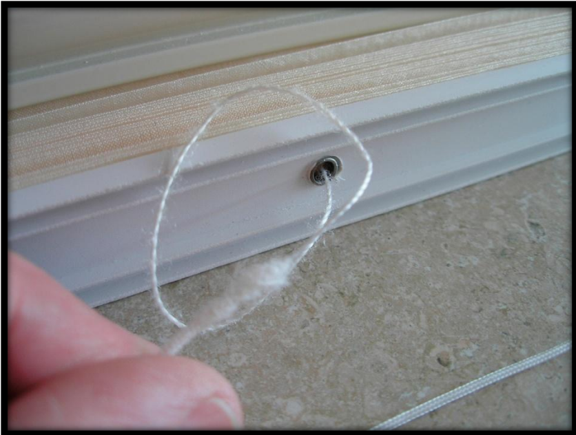
Picture 1 – The eyelet shown is the crimped over part of a 1-piece eyelet installed by the manufacturer. The cord after passing through the top has to pass over this rough part of the eyelet with considerable tension. In every set of blinds with frayed cords this will be found.
