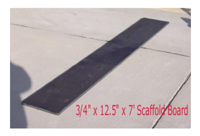
This board was painted on all 4 sides and bottom with gray paint. The top walking surface of the board was painted with Randolph Wing Walk Compound - recommended to make an effective anti-skid surface. This thick paint like compound is available from Aircraft Spruce & Specialty Company in a quart can for \$15.85. Also, you can generally go out to your local airport and get this stuff from an aircraft mechanic.
