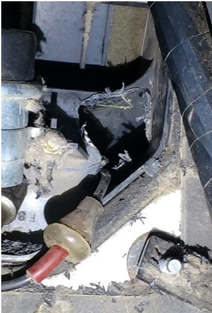
This shows the vacuum line entering the cab with the grommet and red expansion sleeve hanging out of the enlarged hole in the air box. The view is from the passenger side floorboard.
