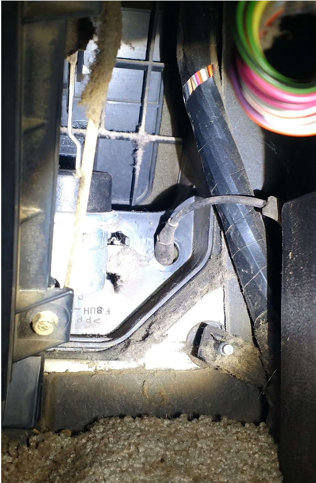
This shows the vacuum line pulled into the cab with the end of the control line attached to the check valve on the other side of the plastic air box. Inspect, but don't disconnect this line.
