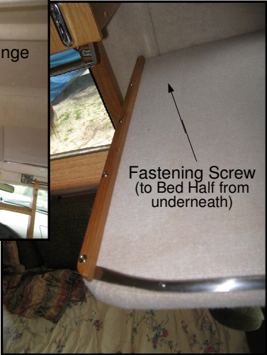
Cushion Retainer (Oak) & Carpet Edge Finishing (SS Boat Rub Rail)
